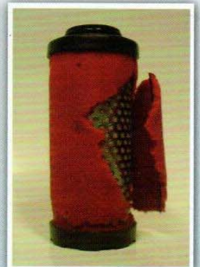
High humidity - Filter damage
