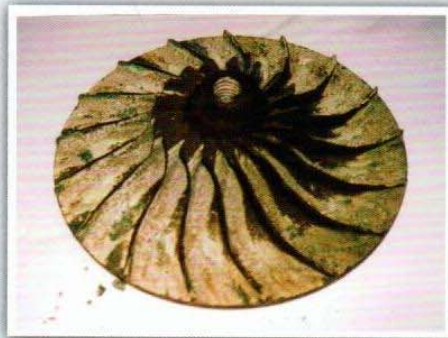
High humidity - Blade corrosion
